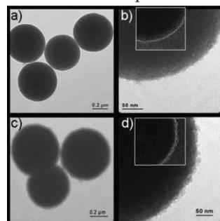
Figure 1: TEM images showing the particles obtained in EtOH at 40 °C in different magnification levels; (a) and (b): after 30 min of reaction, (c) and (d): after 90 min. Inset figures are 'find edge' processed images to reveal the differences in surface of the particles upon reaction time.
