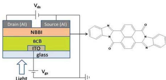
Figure 1. Cross section of device and chemical structure of NBBI.
