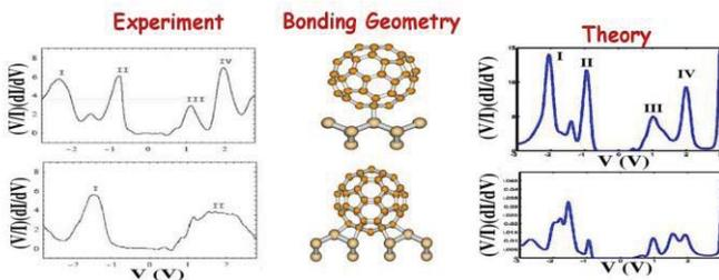
Fig. 2. NEGF-DFT treatment of C60 spectra on Si reproduces experimental variations attributed to alterations in bonding geometry at the interface (adapted from [1]).
