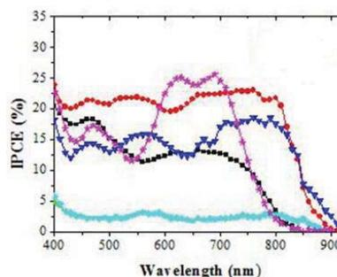
Figure 2. ICPE vs. wavelength data for the series of dyes investigated as a part of this work.
