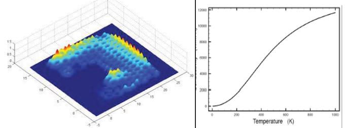
Fig.4. (Left) Computed thermal 'hot spots' in a graphene U-junction, and (right) the bulk graphene thermal conductivity.
