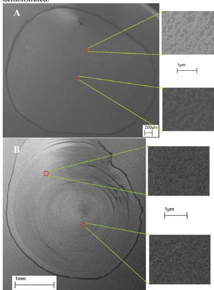
**Figure 1.** Assembly of 200 nm latex nanoparticles from a drying droplet on hydrophobic surfaces (A) and uniform assembly of the same latex nanoparticles upon touching on top of the droplet during its drying (B).
