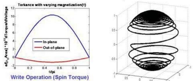
Fig.3. (Left) Computed spin torques, and (right) precession dynamics of free layer in an Fe-MgO-Fe sandwich.
