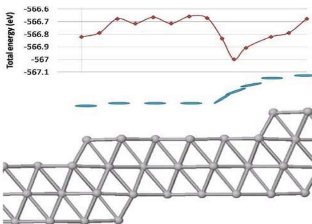
Figure 2. Energetical behaviour of pentacene molecule on Ag(233) surface.
