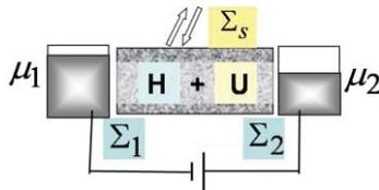
Fig.1. A schematic description of current flow in NEGF
