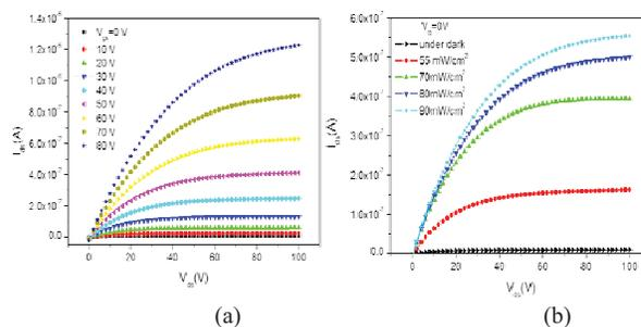
Figure 2. The output characteristics of NBBI based photOFET in dark (a) and under illumination at  $V_{gs} = 0\text{V}$  (b).
