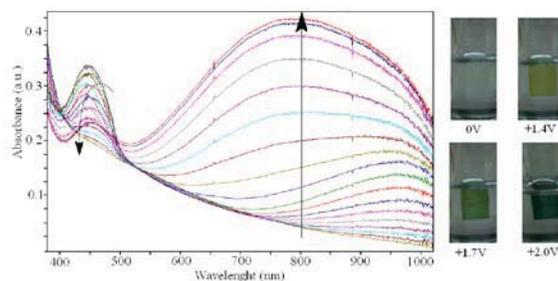
Figure 3. Spectro-electrochemical measurements and color changes of poly-SFC film between 0.0-2.0V.
