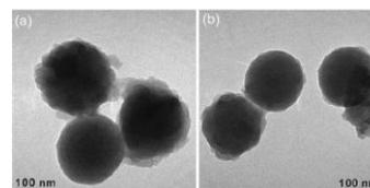
Figure 2: TEM images of PPy-grafted silica nanoparticles on a) silica nanoparticles prepared after 30 min and b) after 90 min of reaction.
