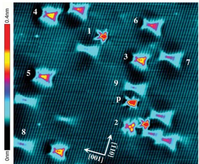
Figure 1: (45nm x 35nm) Constant-current STM topography image of the GaAs(110) surface showing a number of Mn acceptors in their neutral charge state. The numbers correspond with the atomic layer position of the Mn acceptors on and below the GaAs cleaved surface.
