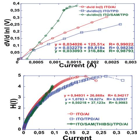
Figure 3. The plots of  $dV/d\ln(I) - I$  and  $H(I) - I$  of the ITO/Al Schottky diode
