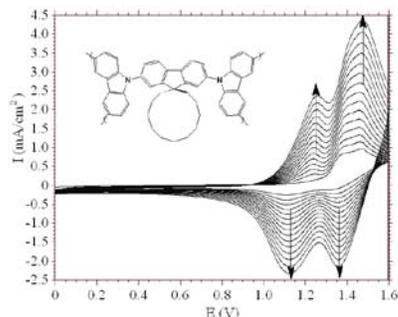
Figure 2. Repeated potential scanning of SFC monomer
