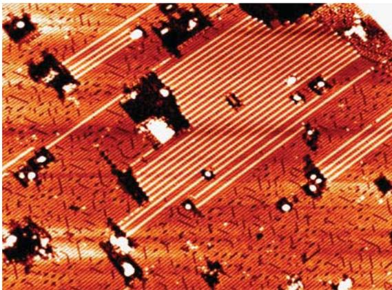
Figure 1. 100nm x 80nm STM image of Ge(001) surface with Pt NWs. Imaging conditions: Sample bias -1.45V, tunneling current 0.41 nA. White linear structures are the individual Pt NWs that are 1 atom thick. Underlying terrace is the beta terrace [1].
