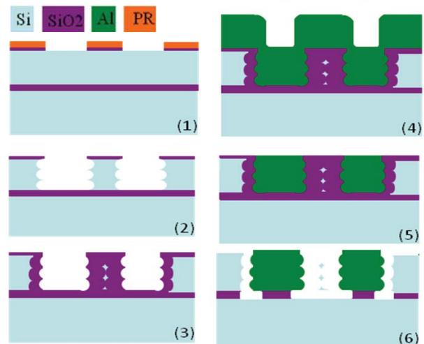
Figure 2. Proposed fabrication flow. (1) Photolithography is carried out with AZ92XX resist, (2) Trenches are opened via Bosch process, (3) Wet oxide growth to attain NWs, (4) Metal deposition, (5) CMP of metal, (6) Silox bath to free the NWs.
