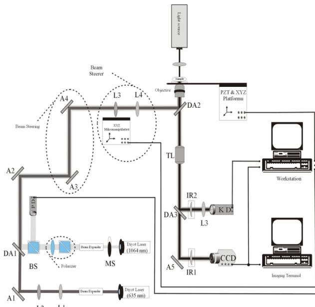
Figure.1 Optical Tweezers layout.
