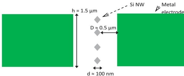
Figure 1. Cross-sectional sketch depicting the Si NW array (grey) present between the metal electrodes (green). NWs are extending in the out-of-page direction. Trench height,  $h$ , diamond-shaped NW width,  $d$ , and NW-electrode gap,  $D$ , are shown.
