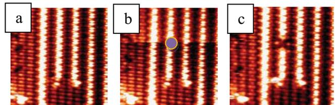
Figure 2. (a) Five Pt nanowires on a beta terrace before manipulation (20 mV, 0.4 nA); (b) during scan, the pecking event is applied on the designated point; (c) rescan of the area after the pecking event; the missing nanowire piece is visible as a dent.
